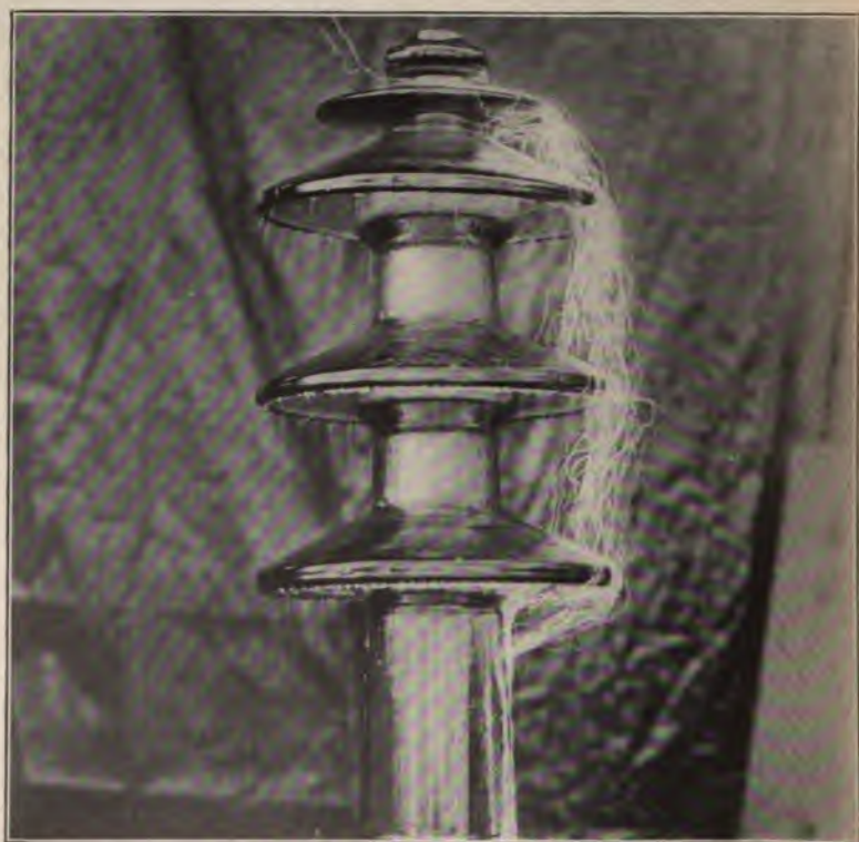
FIG. 13.— EXPERIMENTAL INSULATOR UNDER TEST AT 198 KILOVOLTS.
